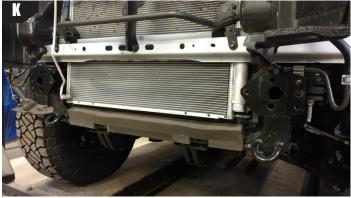
**6)** Remove plastic vertical air dams on each side of the radiator.
