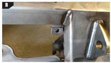
Now bolt the plate on using 4 % x ¾ button head bolts.
