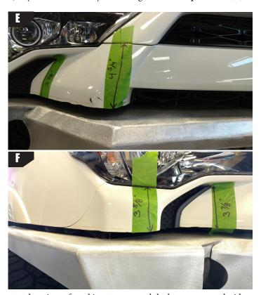
stretch a piece of masking tape around the bumper on each side to middle grill, (a laser can be helpful with this step, they can be found inexpensive at Harbor Freight). **Photo** – **G** shows where to cut the grill. Once the cut is complete the bottom half of the bumper should fall off.
